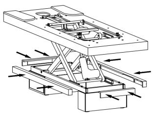
• Insert the armrest in the correct position so that the pin fits with the plastic part of the stretcher body and push it in until the stop.
